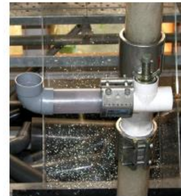
Photo 4: No presence of spouting of water at backflow pipe at 20l/s
